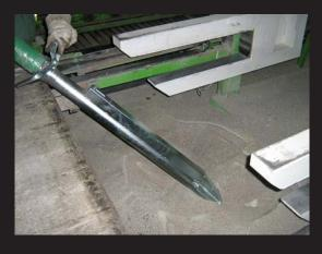
Vacuum extraction of concrete residuals with suction hose DN 80
