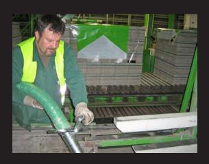
Suction of concrete residuals and cement during the production of precast concrete blocks
