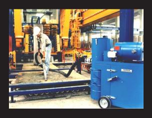
Concrete particles are removed from a product palette
