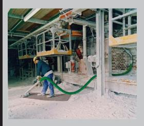
Large quantities of suction material are being extracted with floor cleaning nozzles (surface cleaning) or with secondary air inlet nozzles for larger material accumulations. Flexibel rubber hoses DN 80 are electrically conductive and offer the best compromise between flexibility and resistance to wear.
