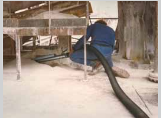
Vacuum extraction of dust and spillages in different production facilities e.g. silo areas.
