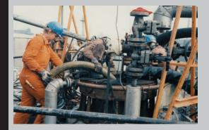
High suction and filter performance during discharge of reactor towers. Suction operation under nitrogen atmosphere. The nitrogen is fed back to the reactor. Suction performance up to 10t/h.
