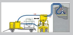
Discharge of a reactor under nitrogen atmosphere. The cooled nitrogen is returned to the reactor.
