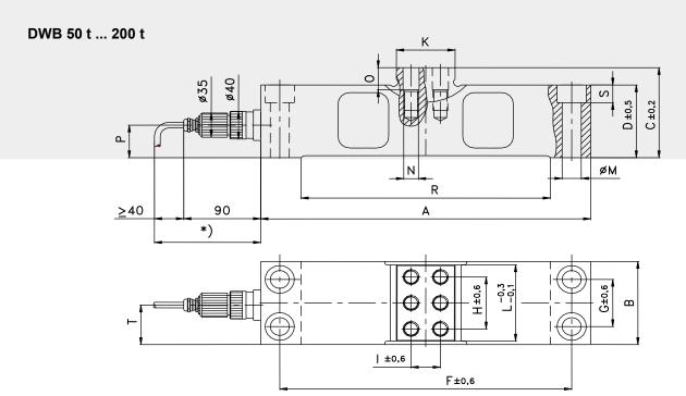
\*) The optional version of the DWB with angular connector requires only 65 mm for the connection plus 15 mm for separating both parts of the connector.
