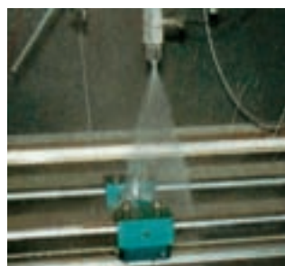
Spray impact measurement device
