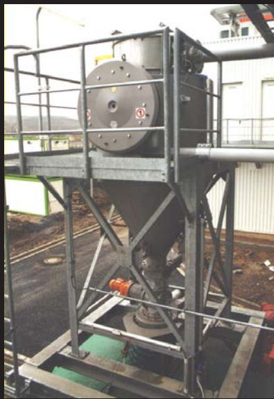
Filter hopper with explosion protection system
