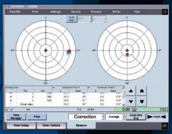
By marking the measured value and averaging over several runs, you can correct the unbalance behavior of unstable rotors.
