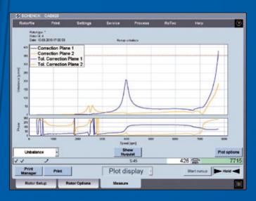
The unbalance effect of a flexible rotor can be measured during start-up displayed in a Nyquist diagram.
