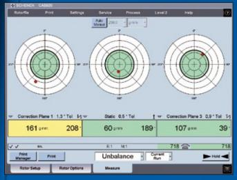
Even in the case of flexible rotors that need to be balanced in 3 planes, the operator only needs to glance at the screen to see the amount and angle of unbalance.
