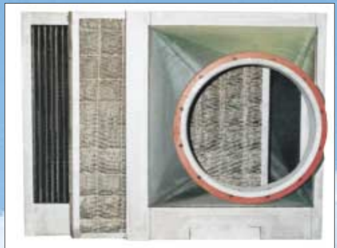
Horizontal gas flow: vane-type separator with agglomerator
