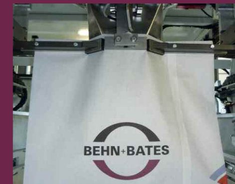
Product-specific: Bag filling by dust-tight powder type spout
