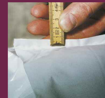
Cost-saving: Reduced film consumption due to minimum weld seam overlaps
