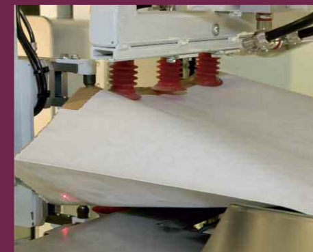
Well-proven: Bag opening by sucker bars
