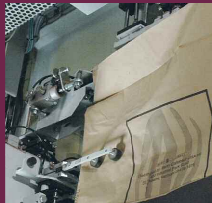
Controlled valve opening for optimum automatic bag application
