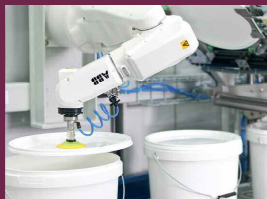
PailFill: Filling of pails – on request, with automatic lid placer
