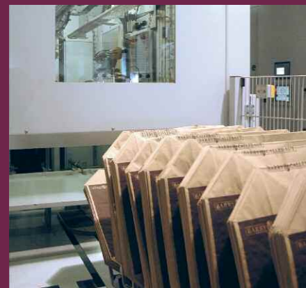
Empty bag feed from the horizontal magazine into the bag applicator
