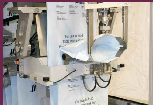
Optimally opened: Shaping of the pre-opened bag for easy application to the filling spout
