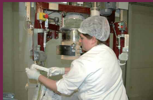
Fixing of the big bag loops onto the slewable hooks
