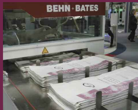
Tailor-made: Empty bag magazine (maximum capacity: 500 bags)
